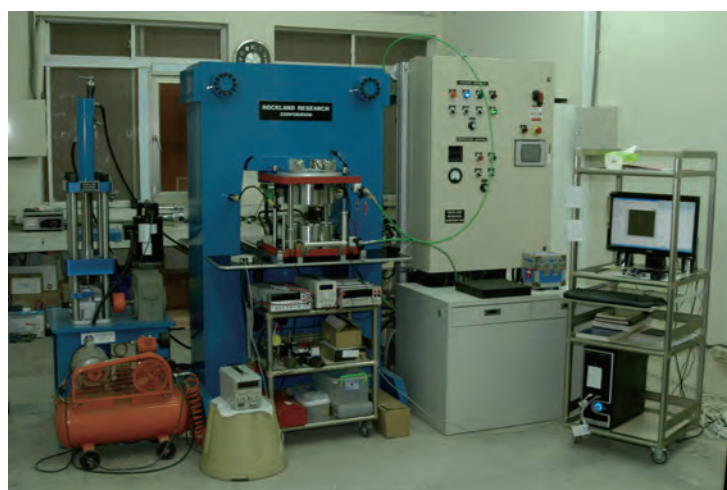
1000 ton press frame with 250 ton D-DIA module and pressure and temperature controlling system.
