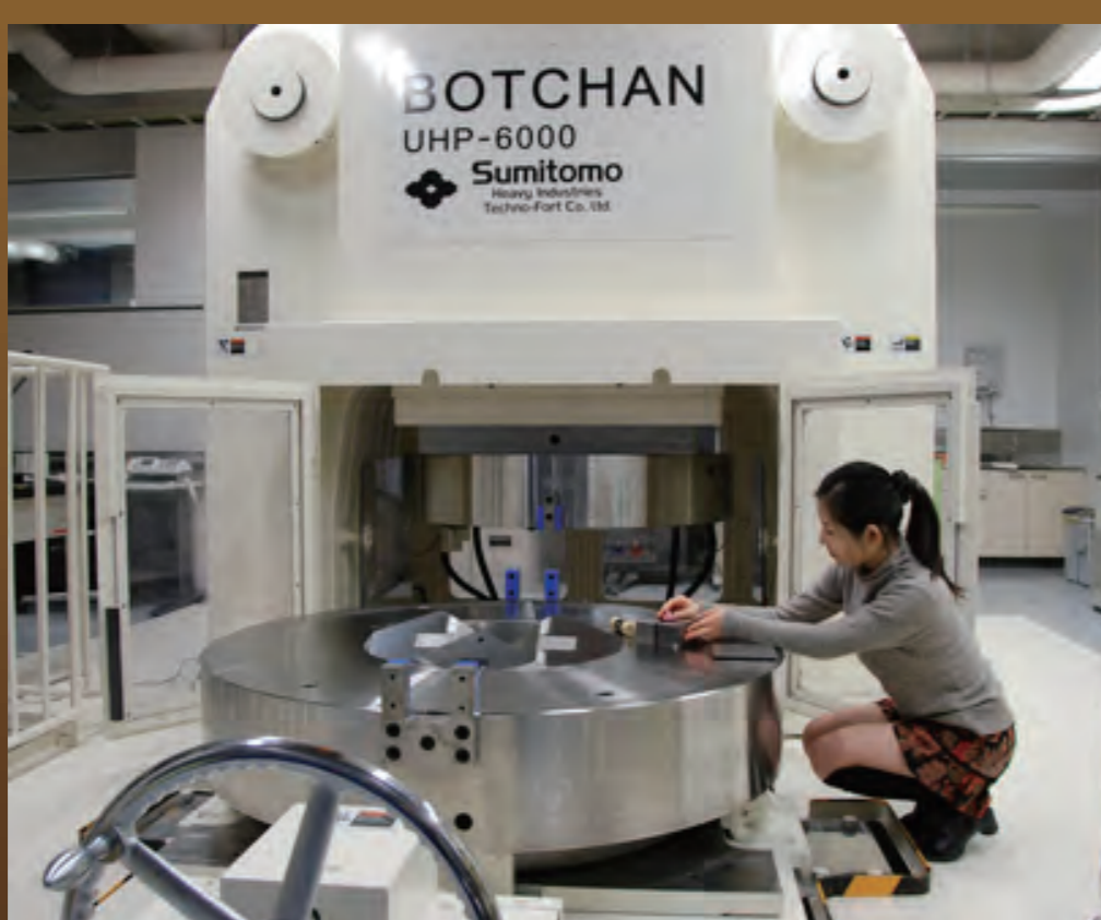
Multi-anvil apparatus (BOTCHAN, the world-largest press, 6000 tons).
