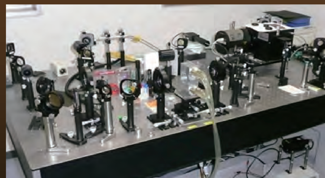
Diamond anvil apparatus: High pressure and high temperature beyond the center of the Earth can be achieved.
